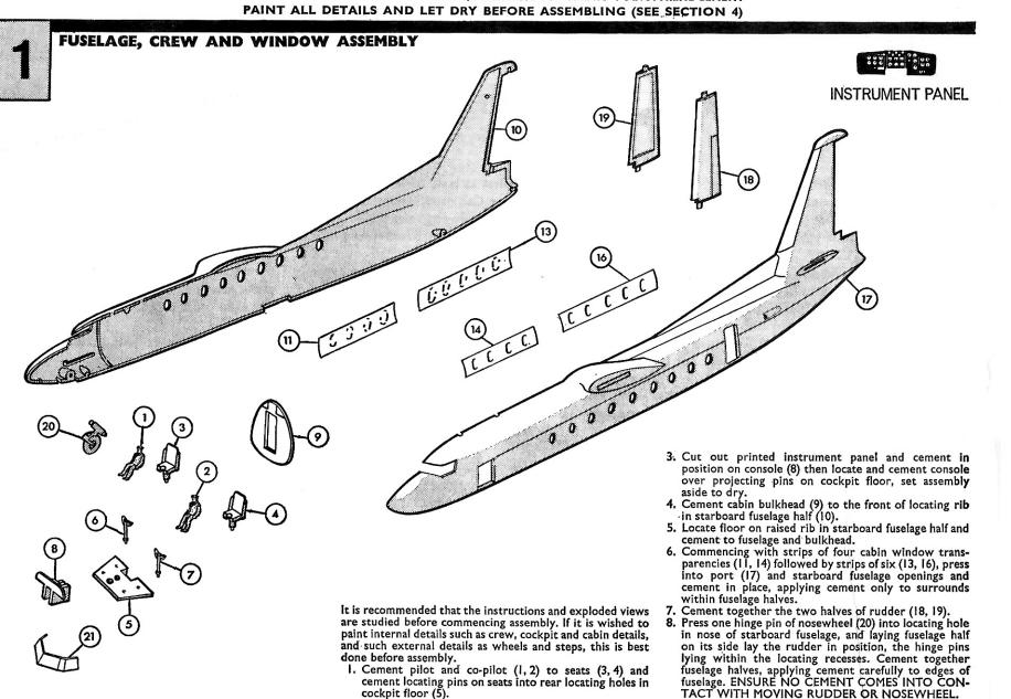
2. Locate and cement control columns (6, 7) into forward
