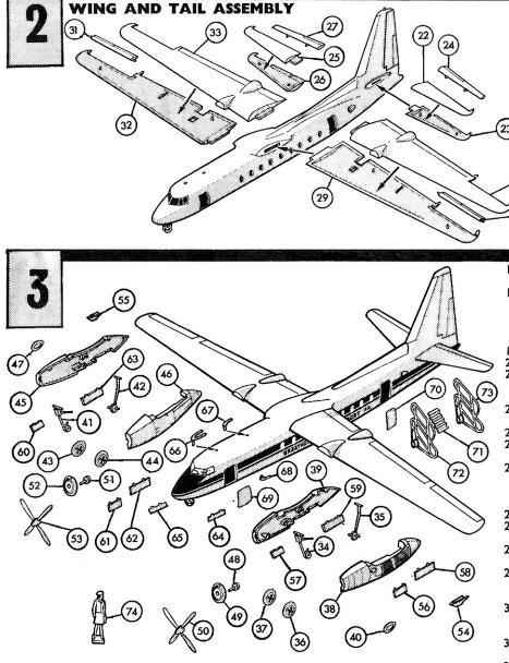
16. Assemble undercarriage legs, note that the two sets of legs are not identical and care must be taken to keep them in their correct relationship, when correctly assembled the front and rear legs will be directly in line. Press axle hole of forward undercarriage leg (34) over the longer axle pin at the bottom of rear leg (35). DO NOT CEMENT.
